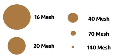
Proppant is shown at scale relative to each size
